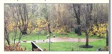
The swale and rain garden have done wonders for the water that used to flood out the yard during heavy rains. When the plants were first installed in the spring, the dirt and mulch would wash away from the swale during storms. The owners patiently repaired the area after each spring storm, and by late summer the root systems had taken hold and made a huge difference in the flooding. The photo below shows the mature rain garden.
